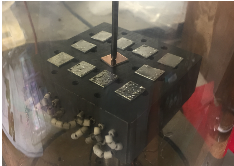
Figure 4.4. A photo of the experimental setup. Since tin melts in the process, the temperature is monitored by the center thermal couple on a bare copper substrate instead of the actual sample.
