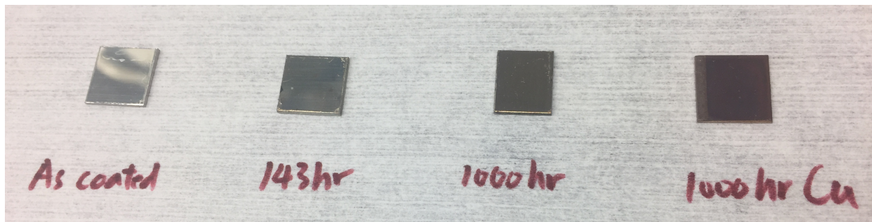
Figure 4.1. A photo of the surface finish comparison of as (Ag)5In coated, 143hr aging, 1000hr aging and bare copper 1000hr aging samples.
