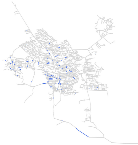
Figure 3.4 Spatial distribution of the pipe damage in the Napa water network following the 2014 earthquake
