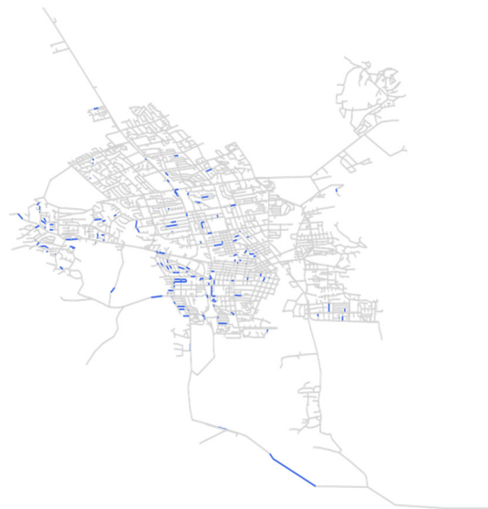
Figure 4.1 Spatial distribution of the pipe damage in the Napa water network in the 2014 event
