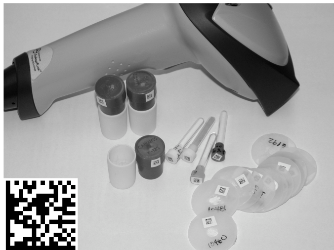
Fig. 4. Alumina crucibles for synthesis, fused silica cuvettes for measuring luminescence spectra and pulsed X-rays, and nylon washers for X-ray diffraction measurements. The hand-operated bar code reader (above) is used to read barcodes shown attached to each sample. Inset (lower left) shows enlarged 2D bar code.
