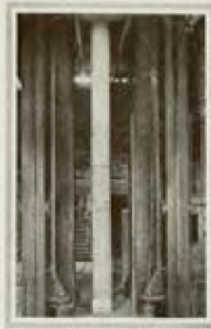
TEST OF A CONCRETE COLUMN The column is 12 inches in diameter and 20 feet long, reinforced with spiral steel wire hooping. Its top is not visible. The testing machine has a capacity of 600,000 pounds and can be used for testing in either tension or compression.
