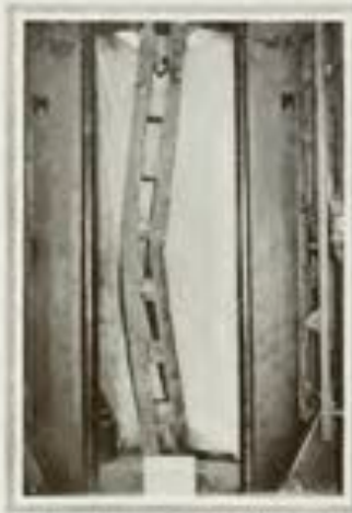
TEST OF A STEEL COLUMN Failure of a built-up steel column made from angles and plates. This type of column is usually imbedded in concrete to give stiffness, and also for fire-proofing purposes.
