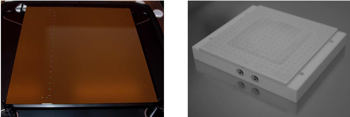
Figure 1.1: Extreme-ultraviolet-lithography mask-chuck system: (left) image of mask by [1]; (right) image of Coulomb-type electro-static pin-chuck by [2].
