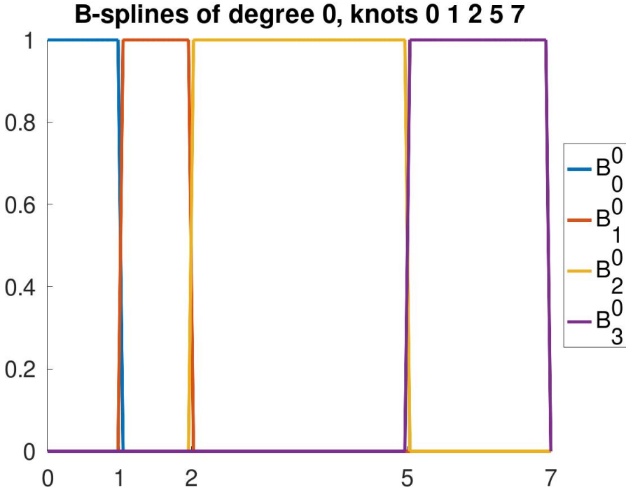
Figure 19: As we can see in this collection of degree 0 B-splines, they are just step functions that are 1 over a single panel and 0 otherwise.
