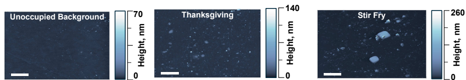
Figure 6.1: 3D AFM height images of the glass surfaces exposed to different activities with scale bars set to 5\ \mu\text{m} . Note height scales increase from 70 to 260 nm across the images of the different activities.
