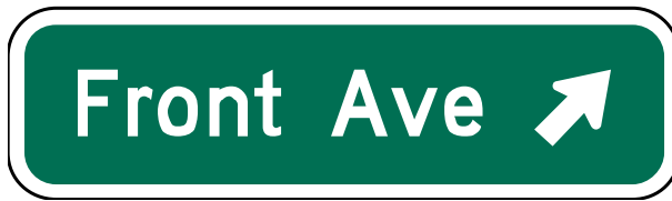
Figure 17: MUTCD Recommended Exit Sign for Roundabouts (FHWA, 2008)
