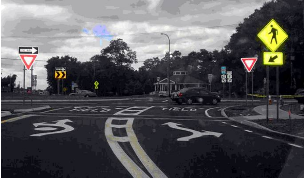
Figure 19: Optional Fish-Hook Lane-Use Arrows (FHWA, 2008)
