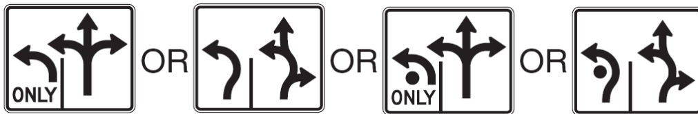
Figure 18: Recommended Optional Fish-Hook Arrows on Lane Use Control Signs at Multi-Lane Roundabouts (FHWA, 2008)
