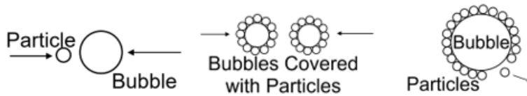
Figure 4.1. Different sub-processes of particle-bubble interaction include particle bubble approaching, attachment, interactions, and detachment a) within the first 5 s, showing a diagram of particle-bubble attachment mechanisms; b) within 20 s, showing a diagram of marble-marble collision mechanism; and c) within 50 s after mixing started, showing marble-marble collision and particle-bubble separation mechanism.
