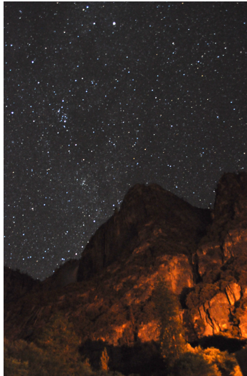
Figure 4.4: Illumination from the candidate light falling upon the cliff face adjacent to the iconic Yosemite Falls. HDRI photography was used to take this image with a thirty second exposure rate.
