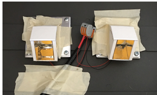
Figure 4.14: Plastic 3D fabricated models implemented in the flood lamp before they melted.
