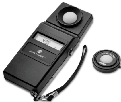
Figure 4.8: Lux meter used in this work. Meter is made by Konica Minolta Sensing Inc. It is the TL-1 model.
