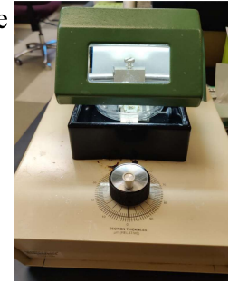
Figure 6: The Vibratome 1000 from Leica as seen in lab and used for all sectioning experiments. Photo taken by me.
