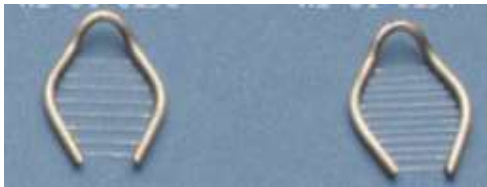
Figure 8: Two harps in the shape designed for RC26G chamber. One is 1mm between each thread, and the other is 0.5mm (Photo taken from https://www.warneronline.com/slice-anchors-kits-harps )
