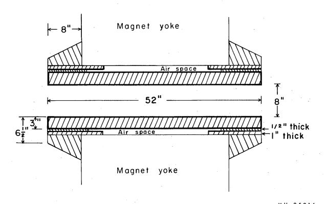
Fig. 7. Spectrometer pole tip and shim configuration.
