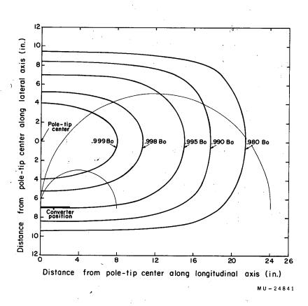
Fig. 10. Magnetic field contours for central field B = 11013 gauss.
