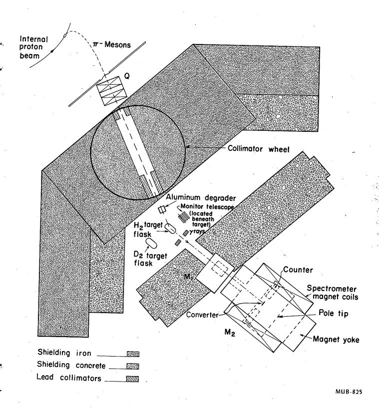
Fig. 2. Equipment set-up in the meson-beam cave of the 184" Synchrocyclotron.
