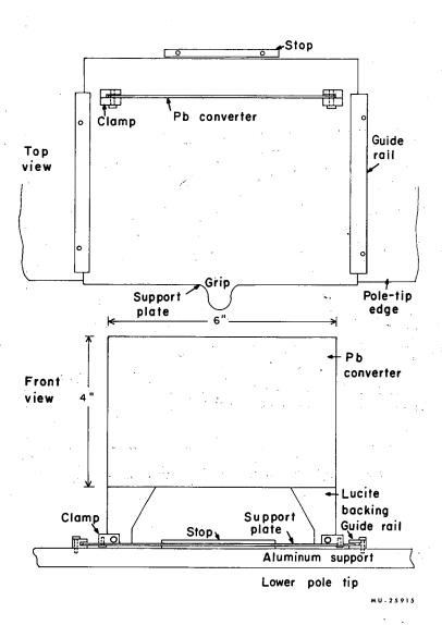
Fig. 11. Converter assembly.
