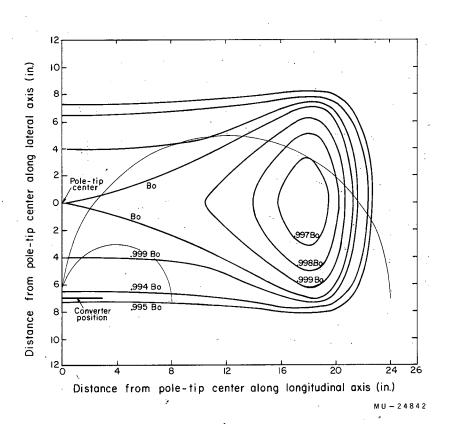
Fig. 8. Magnetic field contours for central field B<sub>o</sub> = 5538 gauss.
