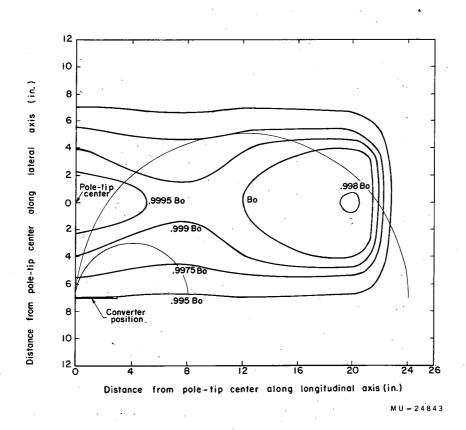
Fig. 9. Magnetic field contours for central field  $B_0 = 10500$  gauss.
