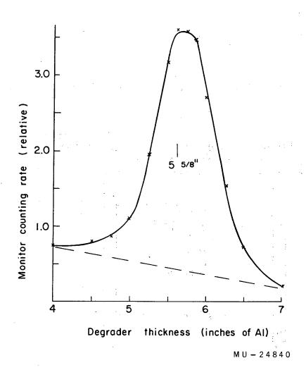
Fig. 3. Monitor telescope counting rate vs energy degrader thickness.
