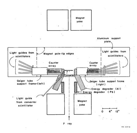
Fig. 6. Top view of spectrometer with upper half of electromagnet yoke removed.
