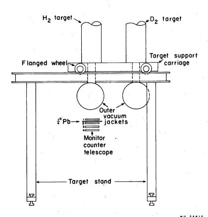
Fig. 4. Schematic drawing showing H<sub>2</sub> and D<sub>2</sub> targets and supporting stand. (Monitor telescope also shown.)
