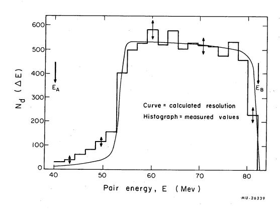
Fig. 21. Mesic capture gamma-ray spectra for B=5,538 gauss.
