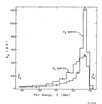
Fig. 24. Measured radiative capture gamma-ray spectra for  $H_2$  and  $D_2$  (B = 10,500 gauss).
