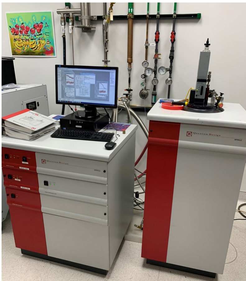
Figure 2.8: Picture of the Quantum Design MPMS XL SQUID Magnetometer in the Lederman Lab at UCSC.
