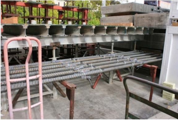
(a) Placing strain gages on test bars
