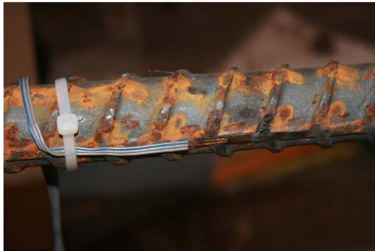
Figure B.2: Strain gage on longitudinal rib of bar
