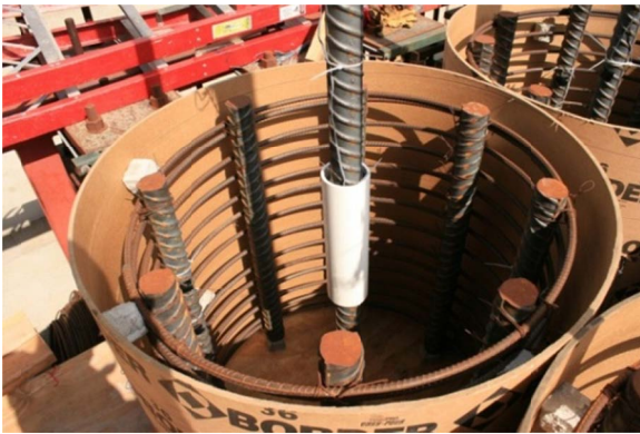
(c) Centering test bar, and placing PVC tubes and form
