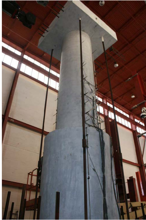
Figure B.23: Column-shaft assembly instrumented (west side)
