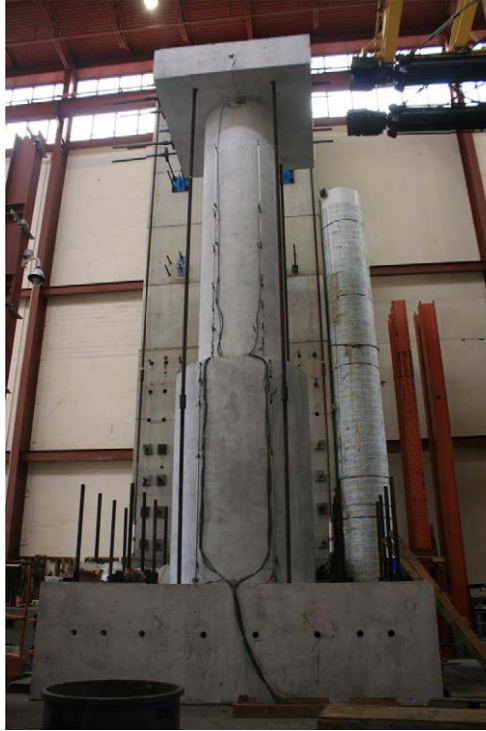
Figure B.21: Column-shaft assembly instrumented (east side)
