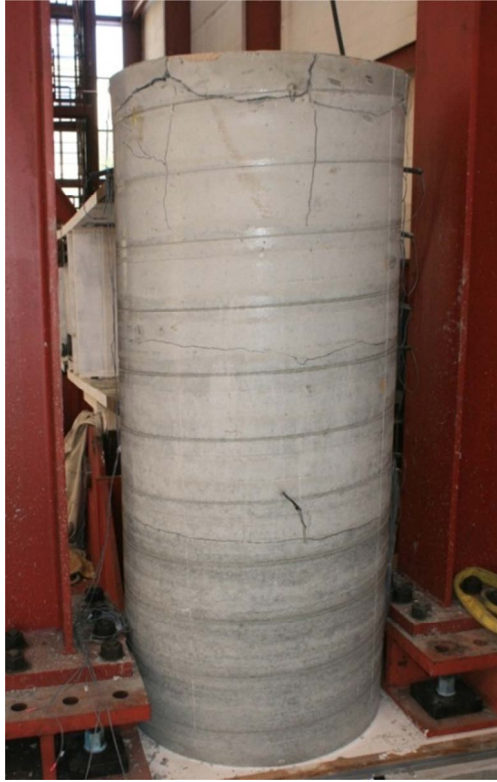
(a) splitting and circular cracks in the concrete cylinder
