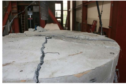
(b) bar fracture and damage atop of the concrete cylinder
