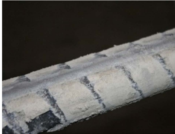
Figure 2.5: Crushing and shearing of concrete between ribs in a bar pull-out failure
