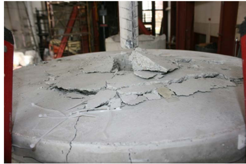
(b) bar pull-out and damage atop of the concrete cylinder
