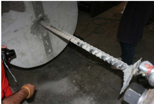
(a) pull-out and cone failure
