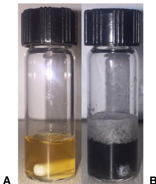
Figure 1: Nanoparticles in aqueous TPGS-750-M solution without NaBH 4 (A) and with NaBH 4 (B)
