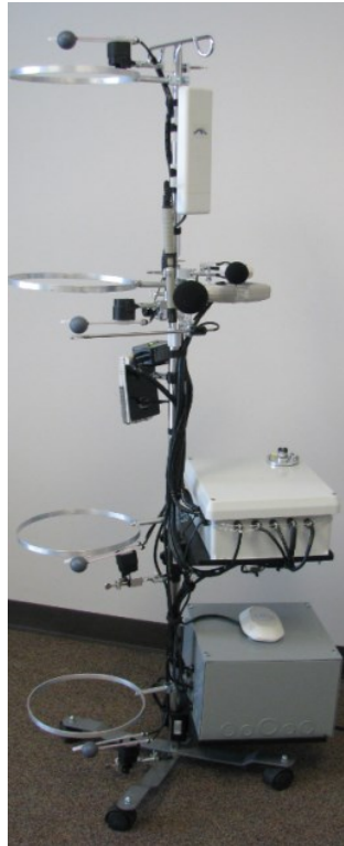
Figure 8: Comprehensive IEQ monitoring cart [37,38]
