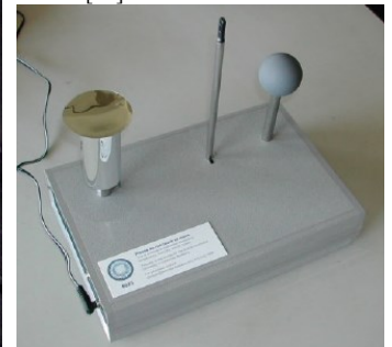
Figure 11: Indoor climate monitor desktop device [40]
