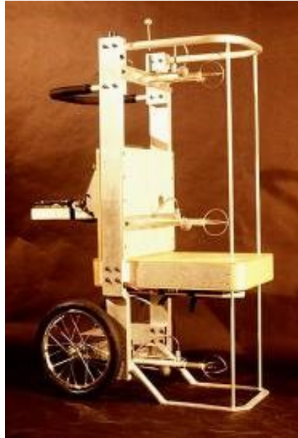
Figure 2: Instrumented chair-like cart [34]
