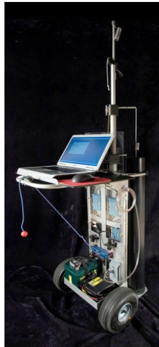
Figure 9: UFAD commissioning cart [39]
