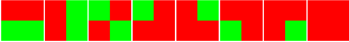
Figure 5.3: Eight 2 \times 2 checkerboard-like filters used in this work. Red (Green) is used to represent value +1 (-1).
