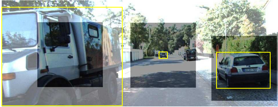
Figure 2.1: In natural images, objects can appear at very different scales, as illustrated by the yellow bounding boxes. A single receptive field, such as that of the RPN [140] (shown in the shaded area), cannot match this variability.
