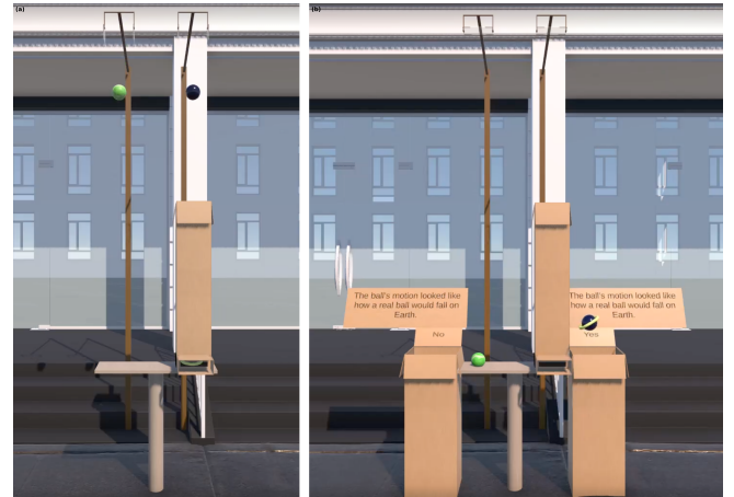
Figure 1: VR setup of Phase 2 (two-ball comparison) . (a) A tall occlusion box is placed on a table directly beneath the falling ball. Participants hold the controller with their dominant hand. The controller is virtually represented as a ring in the VR environment. Participants need to stand closely in front of the table, putting their virtual hand, i.e., the ring, on top of the table and inside the box, and look up to trigger the balls' falling. When they believe that the center of the occluded ball passes the ring, they press the trigger button. They do not see the ring during this catching process. (b) After a delay, the ball comes out from the side of the box, and participants grab the ball to put it into corresponding box that reflects their naturalness judgment.
