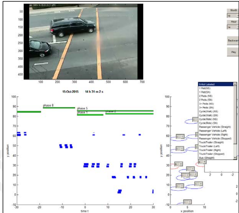
Figure 3.4 Labeling active microradar events
