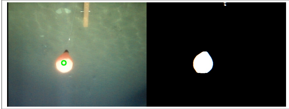
Figure 3.11: Example output using center estimation from area.
