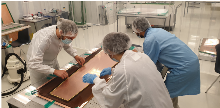
Figure 6.11: The author (left) participating in the assembly of a GE1/1 chamber in a clean room.
