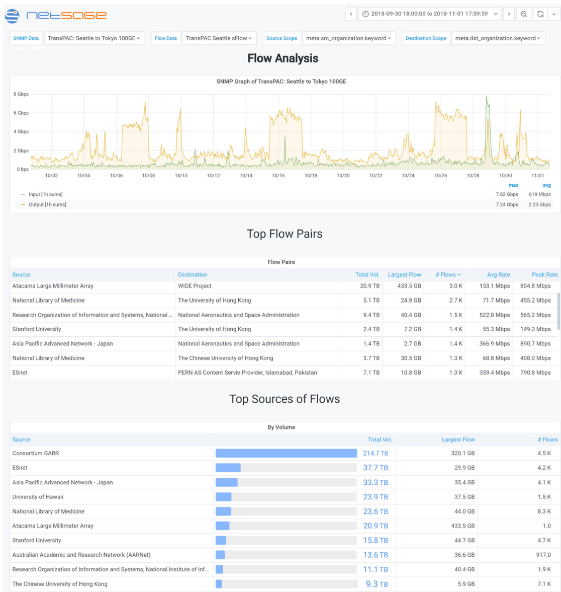
Fig. 16 A partial flow analysis [72] Dashboard showing SNMP and flow data that identifies recurring data transfers that were part of a VLBI astronomy research project between Italy and Japan over the TransPAC4 link between Seattle and Tokyo in October 2018
