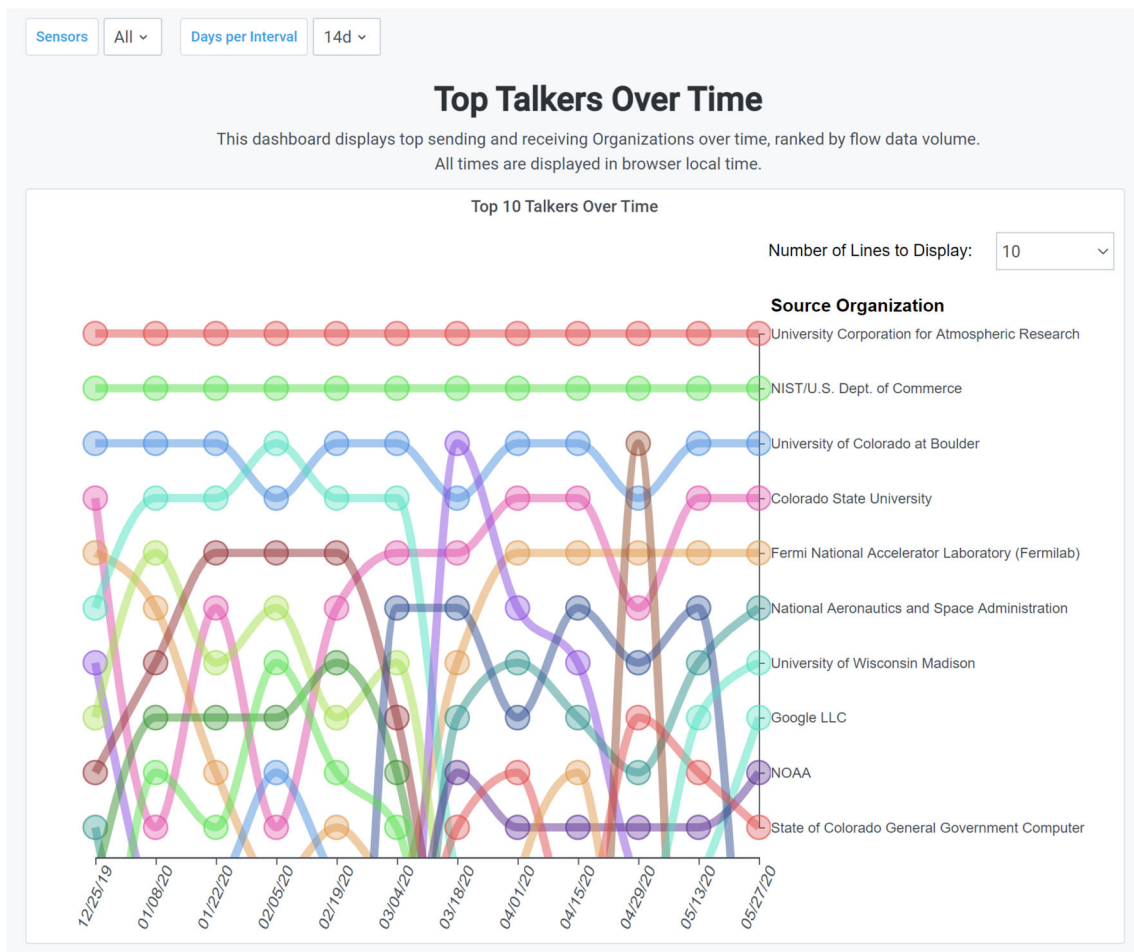
Fig. 10 The FRGP Portal Top Talkers Dashboard for January through June, 2020 [61], showing how the Top Talkers on R&E networks changed radically during the shift in workspace when COVID-19 related restrictions were put in place in early March
