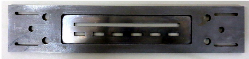
Figure 38: Glue stencil used to apply glue to the backside of a hybrid before mounting it on a sensor. A continuous glue line under all ABC130 ASICs was used to ensure good mechanical support for wirebonding and thermal connection. Alignment holes in the stencil frame allow to position the stencil on the hybrid using the pick-up tool alignment pins.
