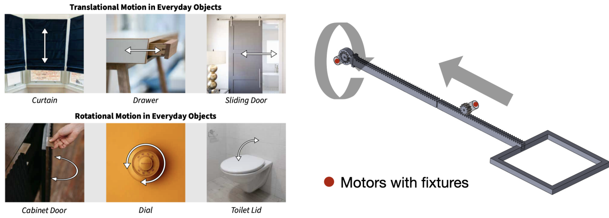
Figure 2.1: Translational and rotational motions are the two common types of motion on everyday objects (left). The device designed to simulate these motions on everyday objects and used in the energy investigation tests (right).
