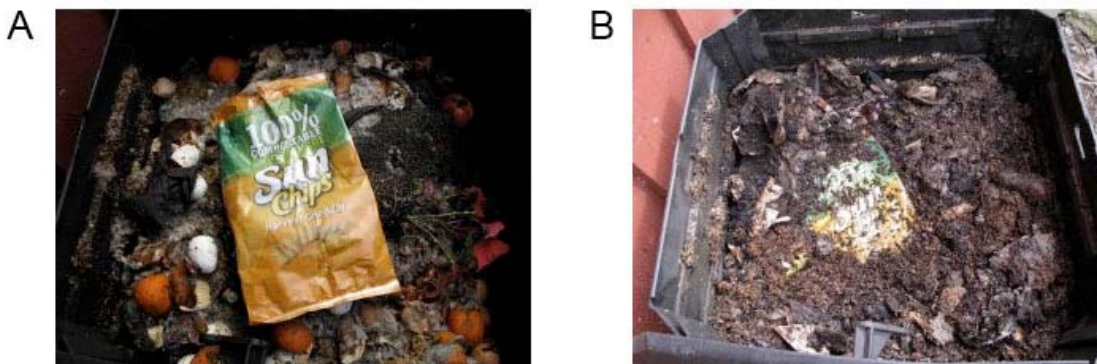
Figure 1.1: Example of a compostable food packaging made from biodegradable polymers. 12 The bag of SunChips® is shown (A) prior to composting and (B) after 18 days of composting.
