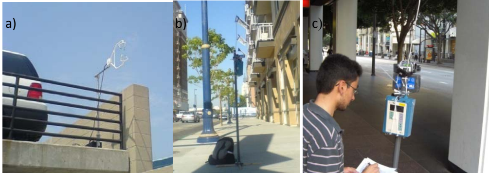
Figure 2.2 a) Sonic anemometer deployed on the parking structure in Long Beach; b) DustTrak on the street in Long Beach; c) DustTrak deployed together with video camera for traffic recording in Los Angeles.
