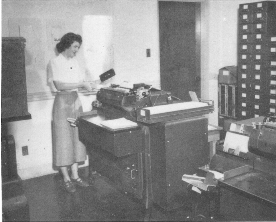
FIGURE 20. One of two model 405 I.B.M. tabulating machines in operation. Photograph by Herb Phillips, San Pedro.
