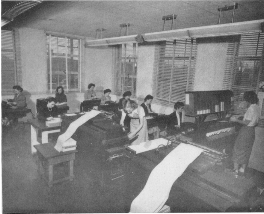
FIGURE 23. The machine room of the statistical unit. The tabulating machine is in the foreground, with the sorter, key-punch and verifying machines against the walls. Photograph by Herb Phillips, San Pedro.
