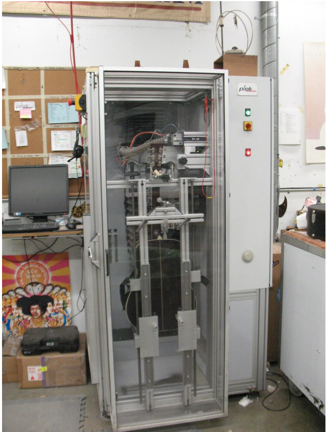
Figure 5 Plek Station, a CNC machine at HT1-1's guitar shop in Hippie Town,
