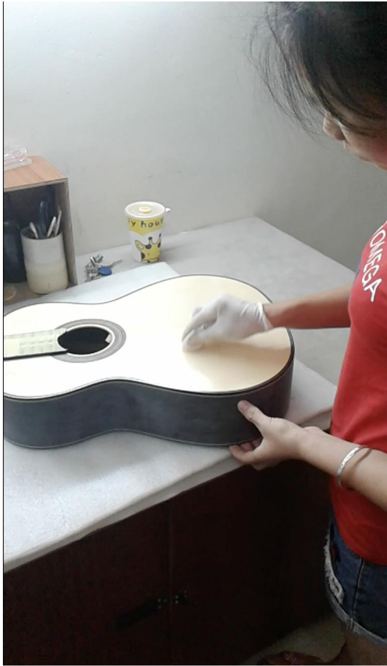
Figure 9 A female worker is finishing a guitar by using shellac
