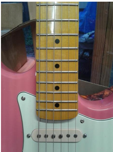
Figure 24 An Installed Pickup on a Fender Stratocaster and its six strings separately suspended above the pole pieces of the pickup
