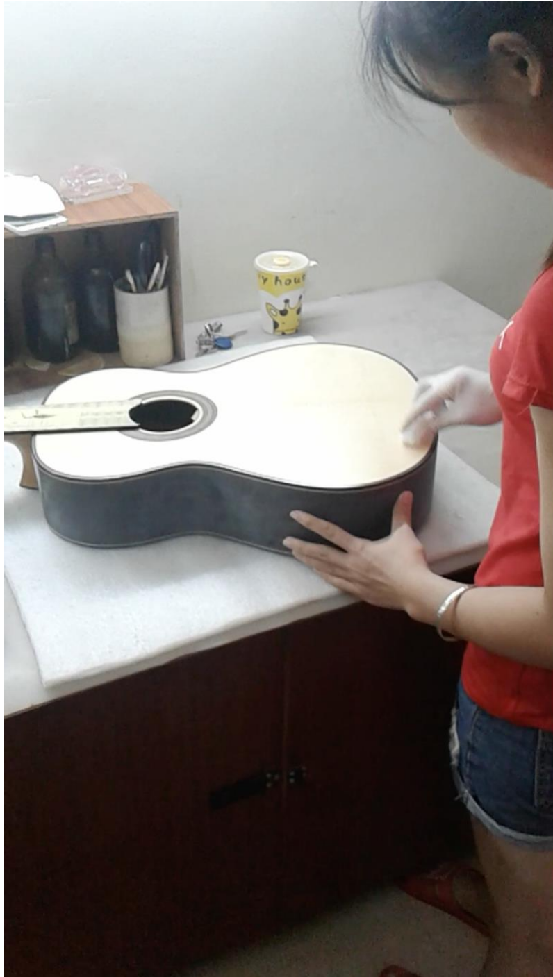
Figure 8 A female worker at MMI Guitars is finishing a guitar by using shellac
