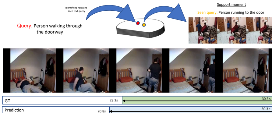
Figure 3.8: Given the text query ‘Person walking through the doorway’ and the corresponding video, our proposed approach retrieves the moment corresponding to the semantically relevant query ‘Person running to the door’ from the train set, reason on that, and identifies the correct moment in the video. GT indicates the ground truth timestamps and Prediction indicates the predicted temporal endpoints of our approach.
