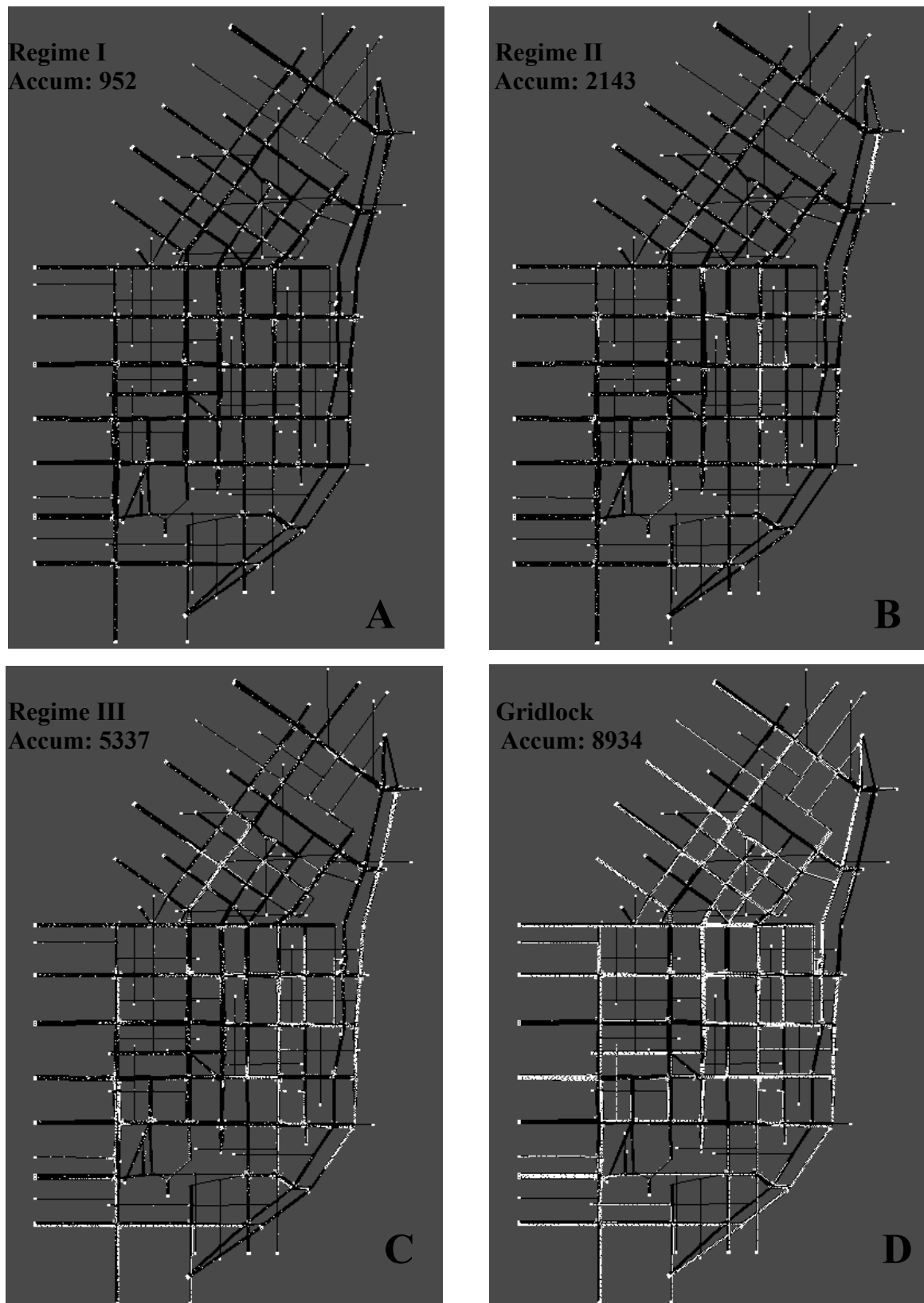
Figure 2.8: Views of the San Francisco network for different traffic regimes (white dots are vehicles; black sections are vacant portions of the pavement)
