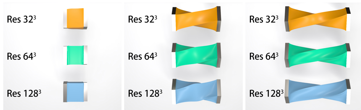
Figure 6.9: Different Mesh Resolution. PBNG produces consistent results when the mesh is spatially refined. The highest resolution mesh in this comparison has over 2M vertices and only requires 40 iterations to produce visually plausible results.
