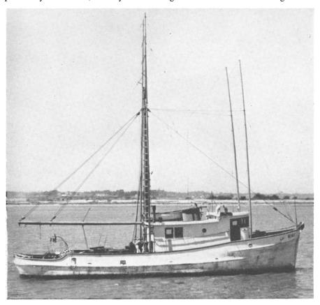
FIGURE 15. Salmon troller. Boats like this carry ice, are capable of long trips, and can follow schools of salmon or albacore anywhere off the coast of California, Oregon or Washington. Four trolling poles, six power operated lines and 24 hooks are most commonly used. Photo by D. H. Fry, Jr., Eureka, California, July, 1948
