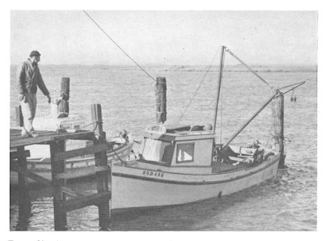
FIGURE 23. A power operated boat with a hoist for handling the large fyke net now in use. Pittsburg, California. Photograph by D. H. Fry, Jr., January, 1949
