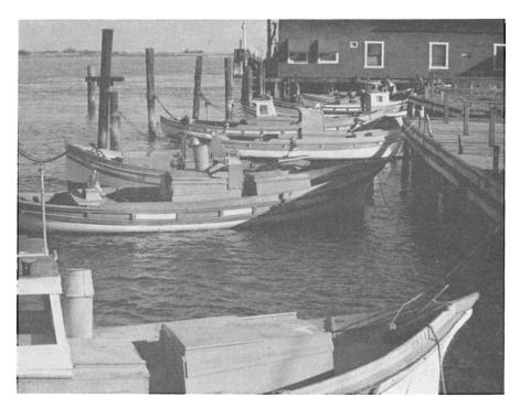
FIGURE 14. Salmon gill net boats. Pittsburg, California. The design is old and standard. Cabins are low to minimize the surface exposed to the wind when the boat is drifting with its net. Radical changes in design are just beginning to enter the fishery. Photo by D. H. Fry, Jr., January, 1949
