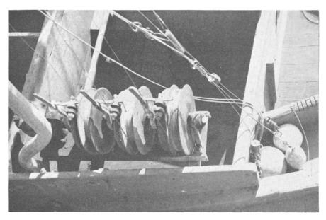
FIGURE 16. Three salmon gurdies mounted on a single shaft. There is a second set of three on the other side of the boat. The lines are stainless steel. Note the three lead weights at the right. Photo by D. H. Fry, Jr., 1949
