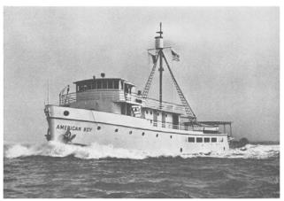
FIGURE 7. A typical modern tuna boat, able to cruise to the equator and back. The entire load of tuna is frozen in
