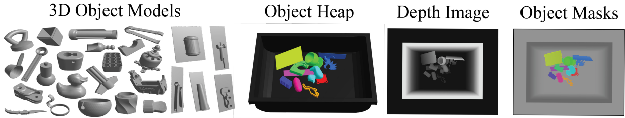
Figure 5.2: Dataset generation procedure for the WISDOM synthetic dataset. A subset of 3D CAD models from a training dataset of 1,600 objects are dropped into a virtual bin using dynamic simulation with PyBullet. A virtual camera captures both a synthetic depth image of the scene and object segmentation masks based on the pixelwise projection of each unique 3D object. This process is repeated to generate 50,000 images.
