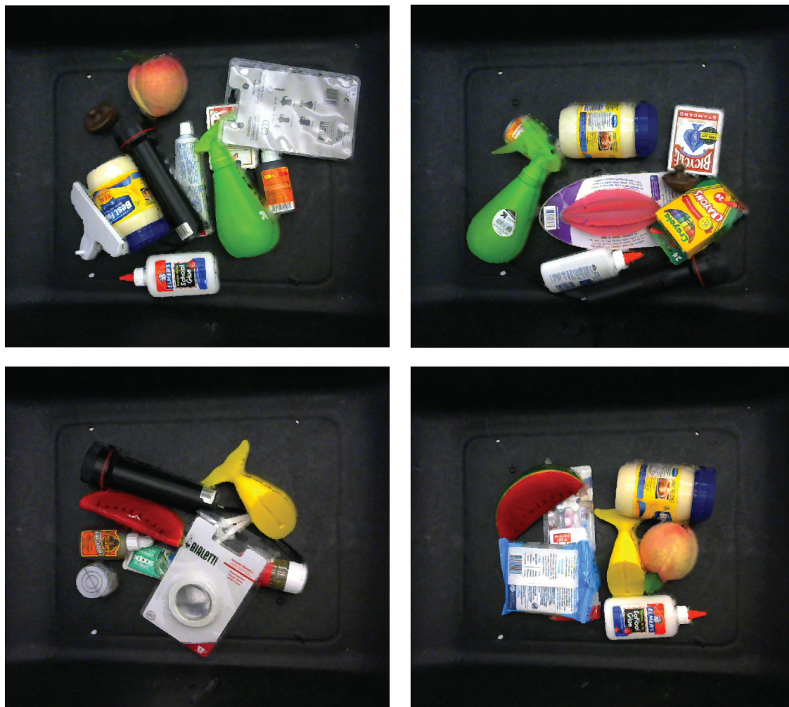
Figure 5.4: Example bins from the WISDOM-Real test set. The number of objects in each bin was chosen from a Poisson distribution with mean 5, with a minimum of two objects per bin. The highly-varied geometry and occlusions make these bins challenging to segment.
