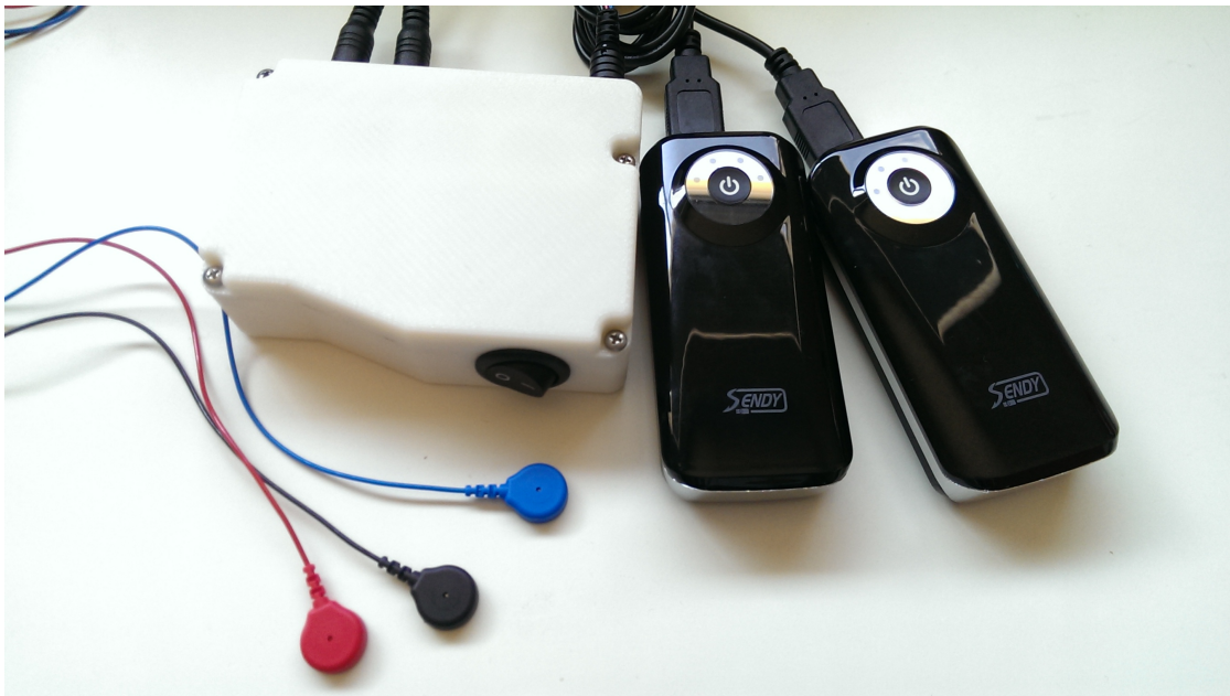
Figure 2.7: EMG unit with two external Sendy 2500mah batteries.
