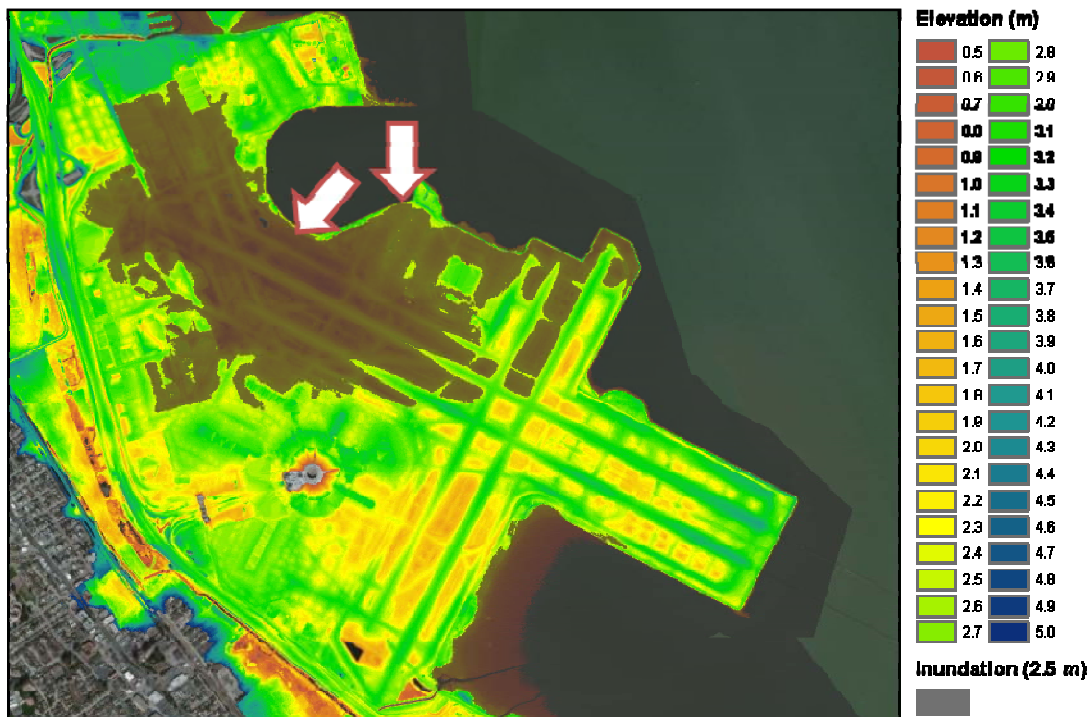
Figure 15. San Francisco International Airport. The potential inundation with the peak water level 2.5 m above the NAVD88 reference datum.
