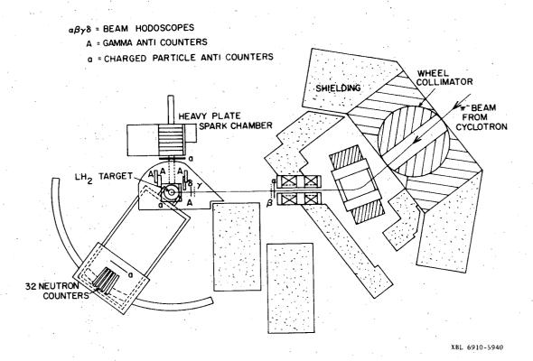
Fig. 1. Beam Layout and Experimental Apparatus.
