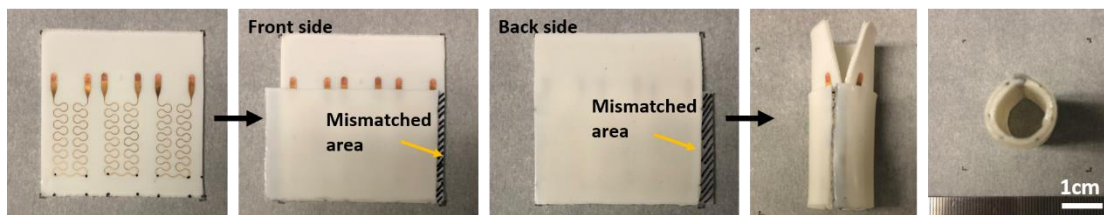
Figure 2.3: Process of the fabrication of an LCE tubular actuator. Three separate heating wires were firstly transferred to a thin LCE sheet. Then, the second layer of LCE sheet was used to cover the three heating wires. Two mismatched areas between the two LCE sheets were intentionally introduced on the edges. These two mismatched areas were bonded to each other after rolling. Finally, the tube was placed under UV light for the second polymerization, and the interfaces of the two layers were bonded through covalent bonds.
