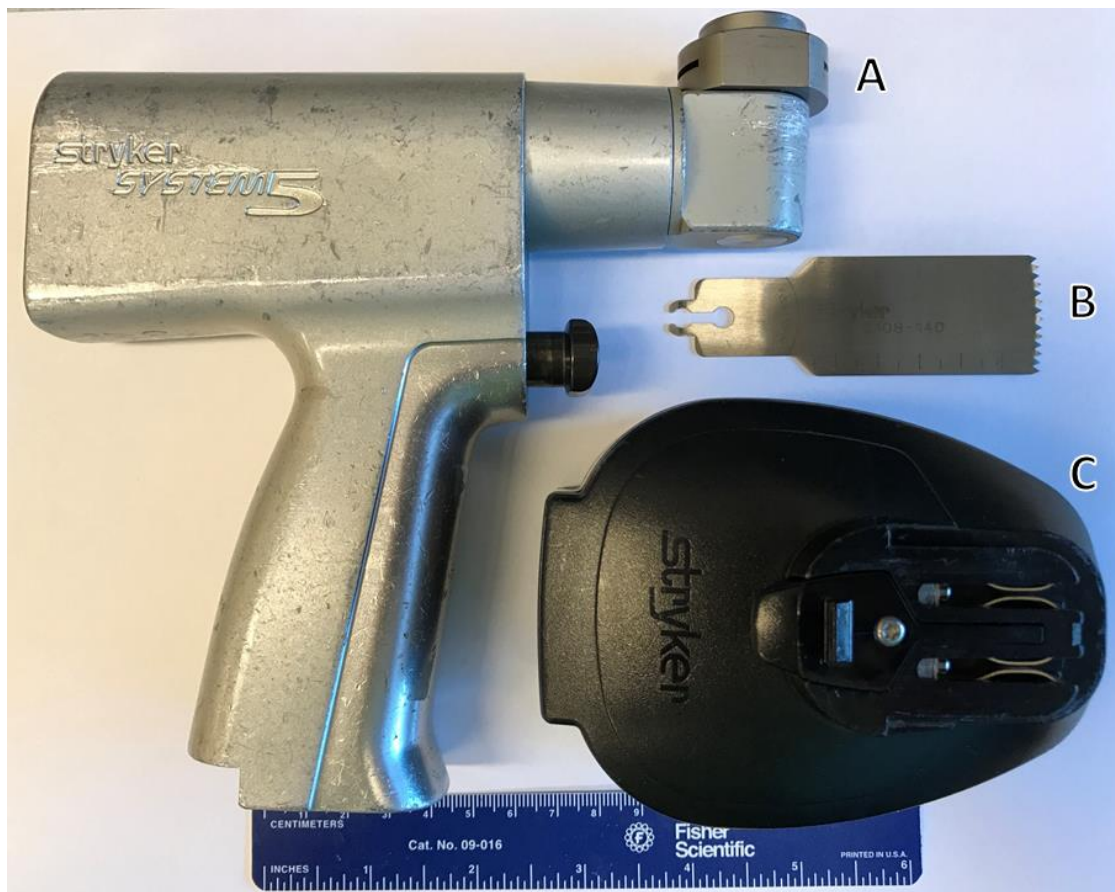
Figure 2.12. Large surgical saw for freeing the donor core from the donor condyle: Stryker System 5 surgical saw driver (A), Stryker 2108-140 surgical saw blade (B) and battery case with rechargeable battery (C).
