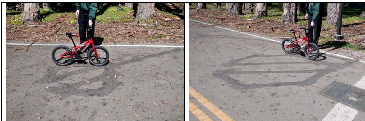
Figure 24 Test Bicycle Aligned with Edge of 3-Foot Type D Loop (left) and 6-Foot Type D Loop (right)
