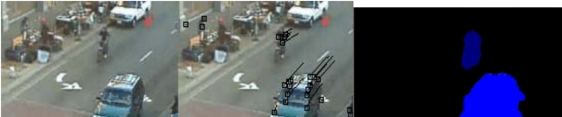
Figure 4 An example image (left); corner feature tracks (middle); and background subtraction blobs (right)
