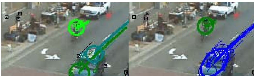
Figure 5 Two-level grouping can be used for varying sizes of objects: cluster-level (left) and object level (right)
