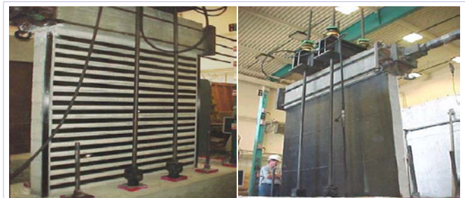
Figure 25: Samples of masonry walls retrofitted with FRP composites: a. Carbon/epoxy procured strips b. Carbon/epoxy wet layup laminates
