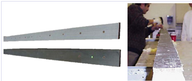
Figure 23: Sandwich composite panels for strengthening wood members.
