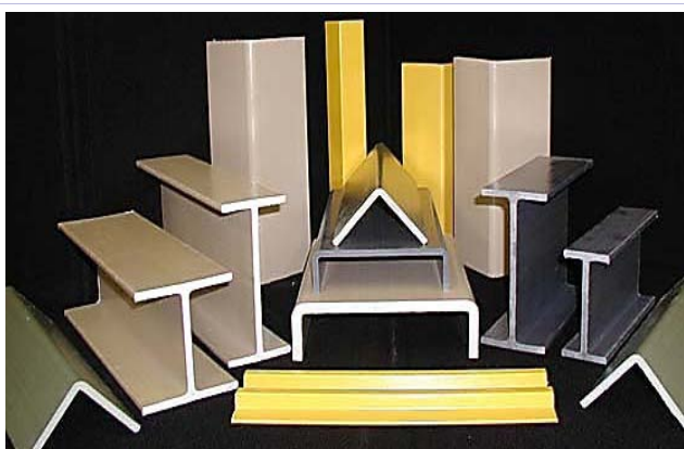
Figure 28: Off-the-shelf pultruded composites.
