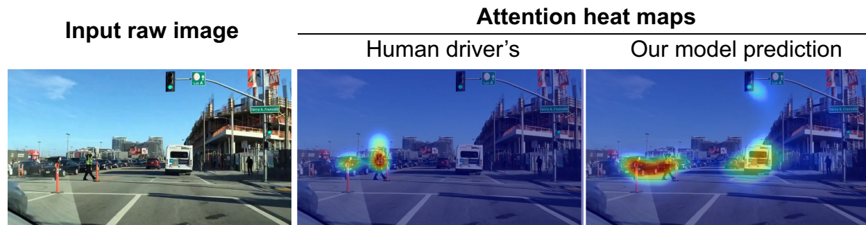
Figure 2.1: An example of input raw images ( left ), ground-truth human attention maps collected by us ( middle ), and the attention maps predicted by our model ( right ). The driver had to sharply stop at the green light to avoid hitting two pedestrians running the red light. The collected human attention map accurately shows the multiple regions that simultaneously demand the driver’s attention. Our model correctly attends to the crossing pedestrians and does not give false alarms to other irrelevant pedestrians
