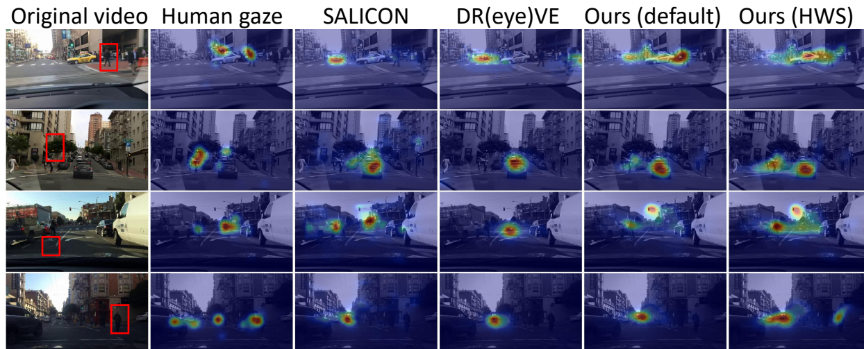
Figure 2.6: Examples of the videos in our dataset, ground-truth human attention maps and the prediction of different models. The red rectangles in the original video column highlight the pedestrians that pose a potential hazard. Row 1: the driver had the green light, but a pedestrian was about to cross the road while speaking on a phone without looking at the driver. Another pedestrian was present in the scene, but not relevant to the driving decision. Row 2: the driver had a yellow light and some pedestrians were about to enter the roadway. Another pedestrian was walking in the same direction as the car and therefore not relevant to the driving decision. Row 3: a cyclist was very close to the car. Row 4: the driver was making a right turn and needed to yield to the crossing pedestrian. Other pedestrians were also present in the scene but not relevant to the driving decision
