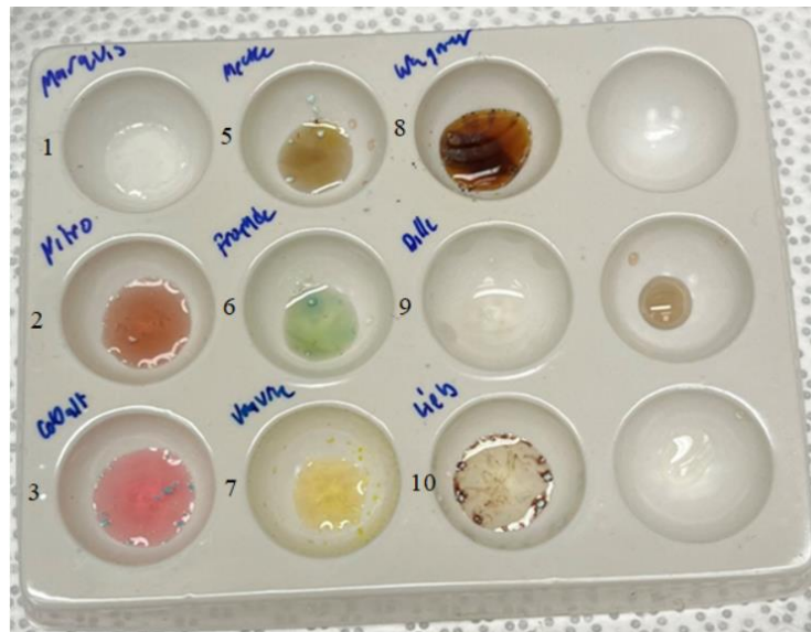
Figure 42 F13 color tests. 1= Marquis, 2= Nitroprusside, 3= cobalt thiocyanate, 4= ferric chloride (not shown), 5= Mecke, 6= Froehde, 7= Van Urk, 8= Wagner, 9= Dille-Koppanyi, 10= Liebermann's.
