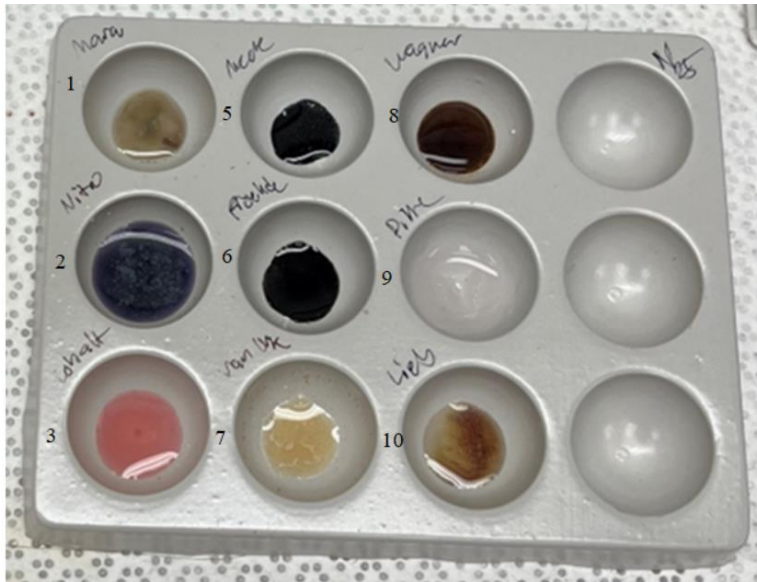
Figure 41 N25 color tests. 1= Marquis, 2= Nitroprusside, 3= cobalt thiocyanate, 4= ferric chloride (not shown), 5= Mecke, 6= Froehde, 7= Van Urk, 8= Wagner, 9= Dille-Koppanyi, 10= Liebermann's.
