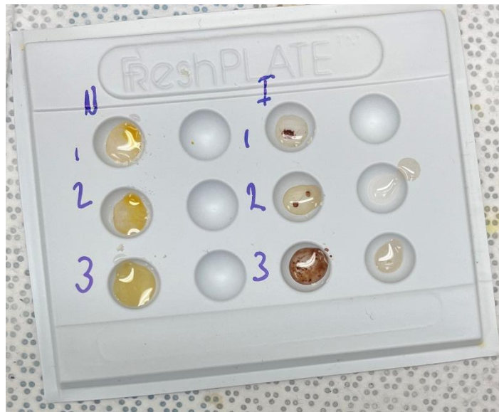
Figure 9 Liebermann's test for nitazene citrate and isotonitazene. N is nitazene citrate and I is isotonitazene.
