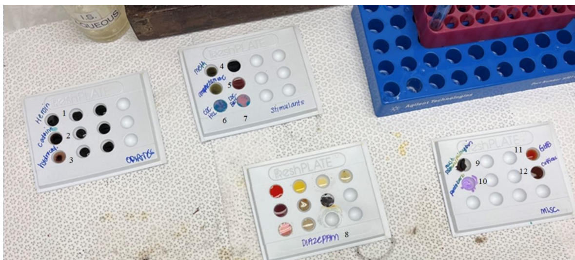
Figure 6 Positive controls for known drugs: 1= heroin, 2= codeine, 3=hydrocodone, 4=methamphetamine, 5=amphetamine, 6= cocaine HCl, 7=cocaine base, 8= diazepam, 9= psilocybin, 10= pentobarbital, 11= GHB, 12= caffeine.
