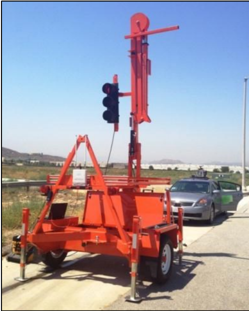
Fig.5.10. Portable Traffic Signal Trailer used in the Riverside field study.
