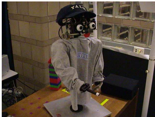
Figure 1: Nico is an upper-torso humanoid robot with the arm and head kinematics of a one-year-old.
