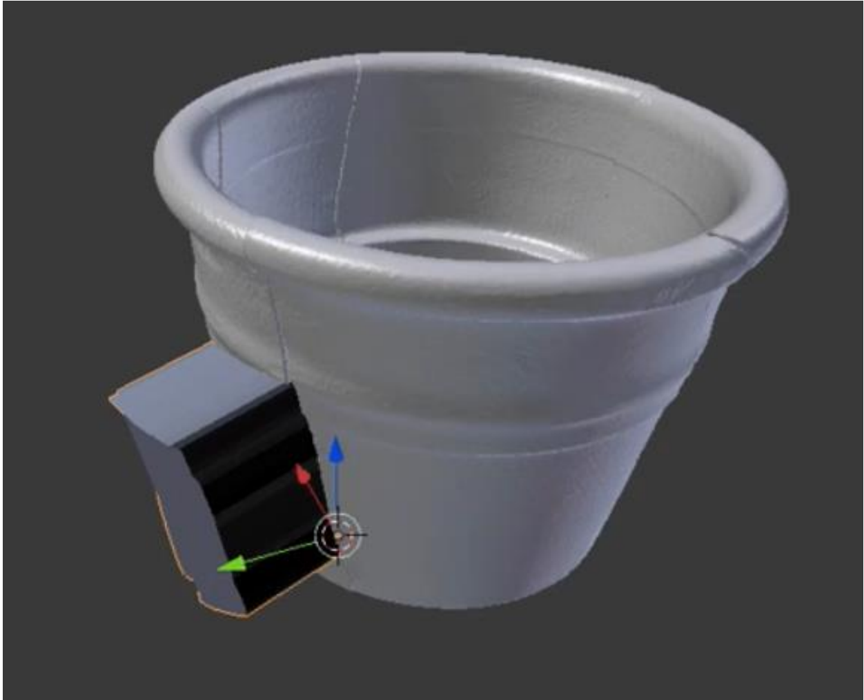
Figure 27: The new cylinder is extruded on the interior and exterior (visible here on the exterior). From this point, the mesh for the “new sherd” is cut out by overlapping an existing sherd and applying a Boolean Modifier.
