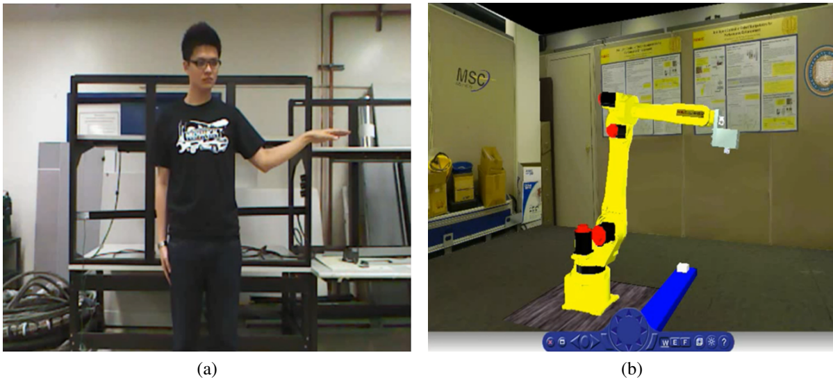
Figure 3.4: Simulation result of robot imitation kinematic control on M-16iB. (a) Human motion capture from Kinect. (b) FANUC M-16iB Visualization in the simulator
