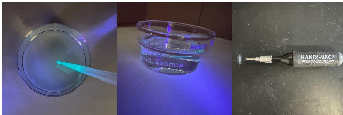
Figure C.3. Photos showing (a) the addition of nanoplate suspension onto GTA sublayer, (b) covered petri dish during evaporation of native solvent, and (c) coverslip vacuum tool used to aid in the even stamping of glass onto the liquid sublayer.
