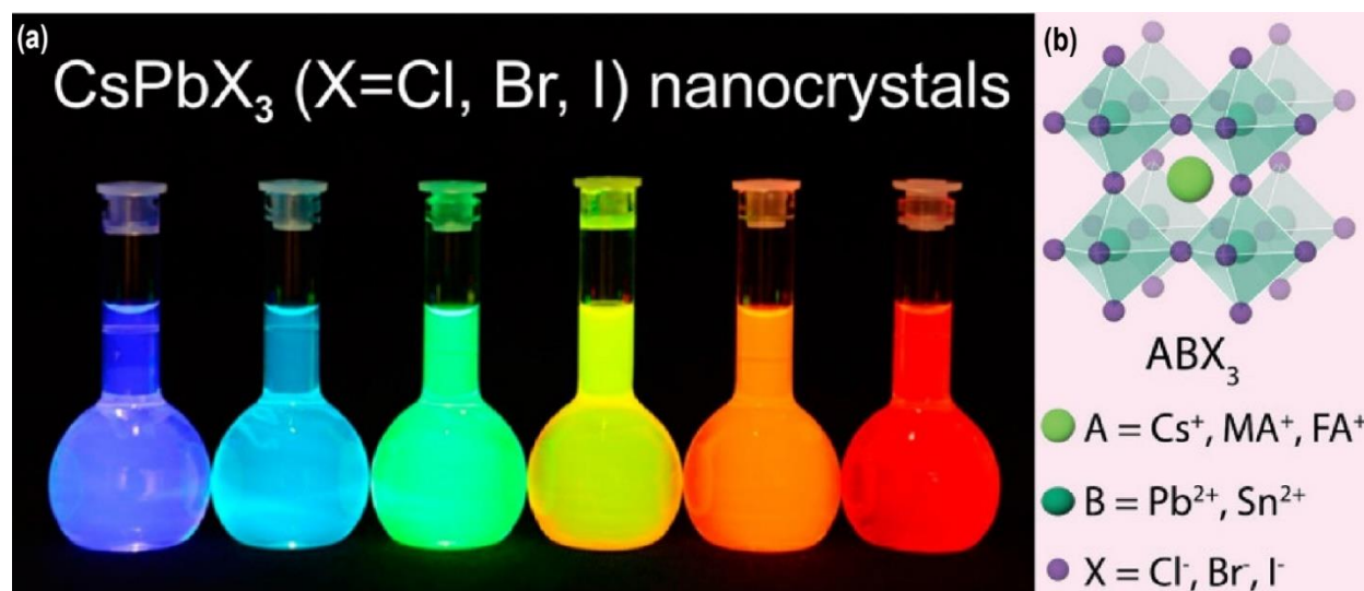
Figure 1.1. (a) Perovskite nanocrystals across the visible spectrum. Adapted from Protesescu et al. 17 (b)
