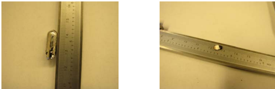
Fig 2.2 Bulk crystal of \text{Bi}_2\text{Se}_3 . The method of preparing the crystal is discussed in the paper Z. Wang Appl. Phys. Lett. (2010) 32
