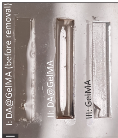
Figure S6.4. Digital photograph of the polydimethylsiloxane (PDMS) molds used to crosslink rectangular (25 mm \times 4 mm) samples. I: Crosslinked dopamine (DA)@GelMA before removal, II: DA@GelMA and III: GelMA samples after removal. Some degree of pre-polymer residue are left behind when DA is added to the hydrogels. Scale bar = 2 mm.
