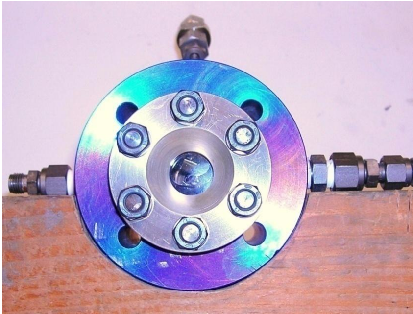
Figure 2-5. A photo of sealed autoclave
